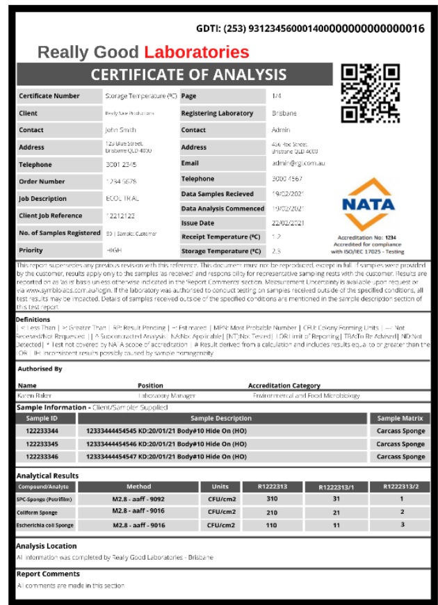
Figure 4: Example of GDTI (top-left) being used for a Certificate of Analysis document type. It is in both a human-readable format and as a machine-readable GS1 QR Code.
